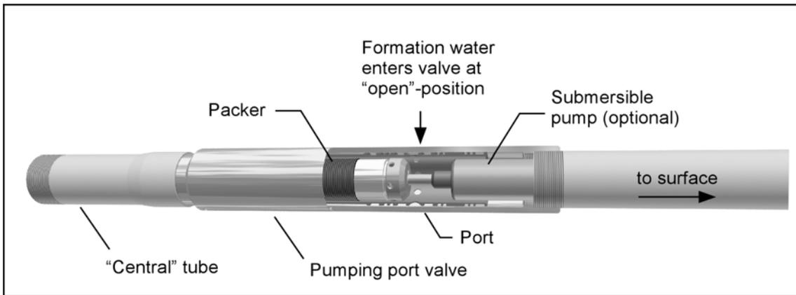
Figure 2: Pumping port valve in "central" tube shown with valve open/close packer.
