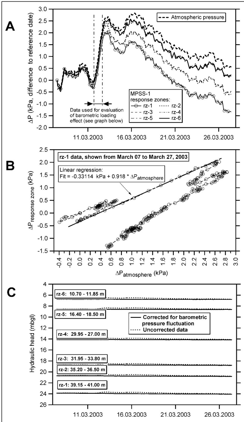
Figure 3: Pressure data and calculated heads from the MPSS-1 system, Whitechapel. The effects of barometric pressure fluctuations (A) are analyzed using a data set that is not disturbed by "artificial" activities (B). Calculated hydraulic heads are shown in graph C. The location of the response zones rz-1 to rz-6 are given in meters below ground level (mbgl) in graph C.
